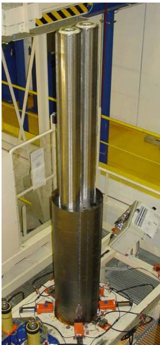
Figure 1: Yoke assembly around quadrupole apertures
