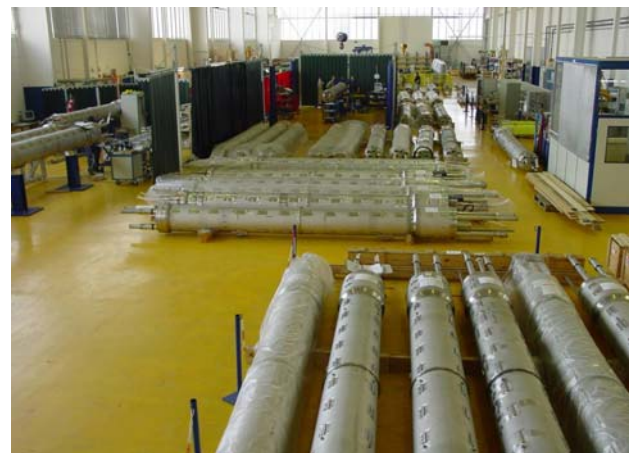
Figure 2: Quadrupole cold masses awaiting shipment at ACCEL
