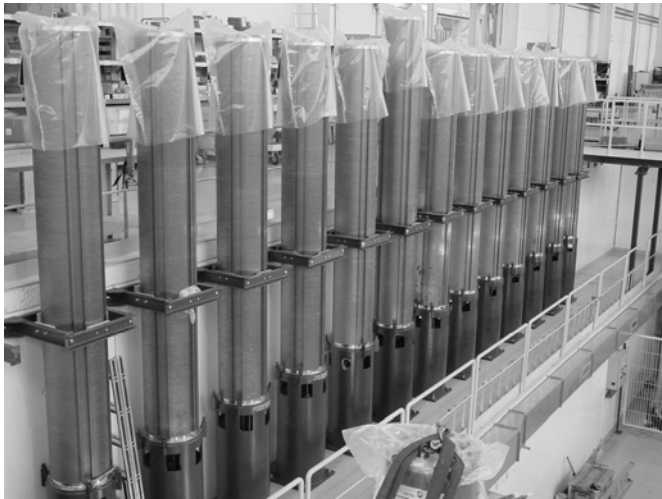
Fig. 4. Finished quadrupole magnets awaiting assembly into cold masses.
